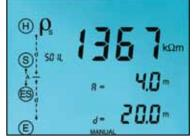
The Schlumberger test displays test lead connection, soil resistivity ( $\rho$ ) test results and electrode spacing.
