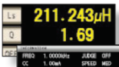
L and Q display screen (1 kHz 1 mA constant current measurement)
