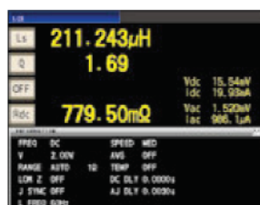
L, Q and Rdc continuous measurement screen
