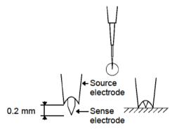
Hold these leads lightly against the two sides of the item to be tested.
